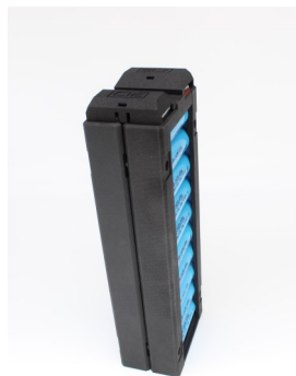
Snap Lock interconnect covers for touch safe operation
